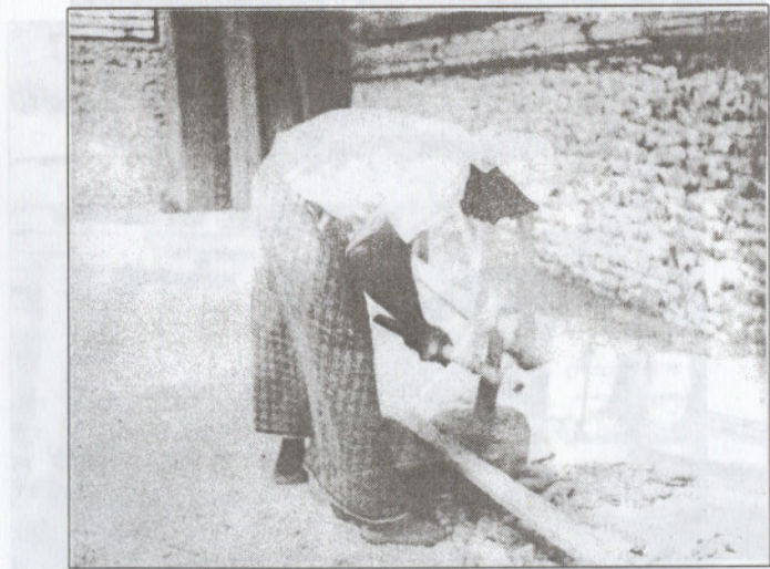
22. Maldivian axe, the carpenter is producing a new oar loom from a coconut plank.
